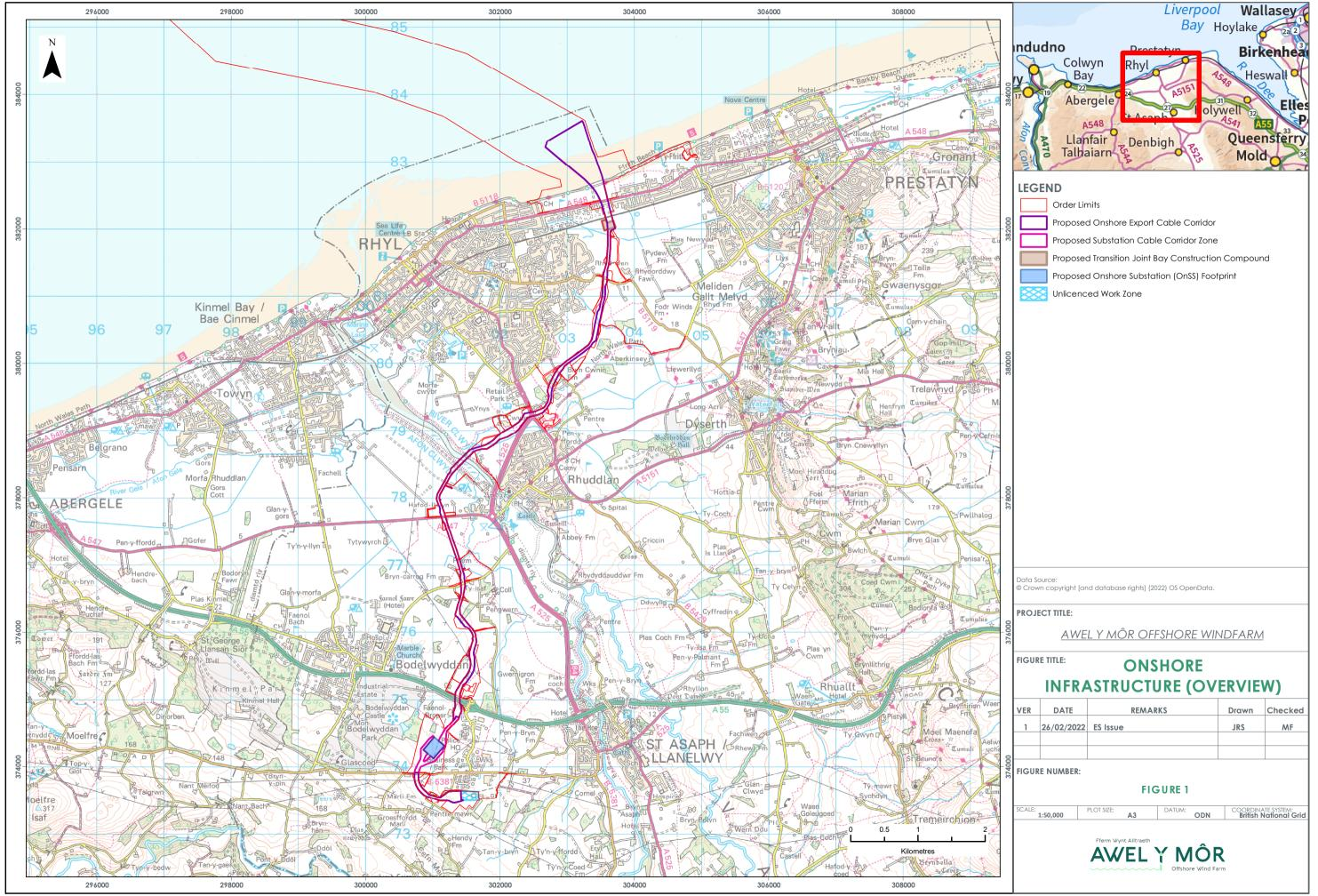
17 The transmission voltage will be up to 400 kV, and the onshore ECC will be approximately 12 km in length from the TJBs to the existing National Grid Bodelwyddan substation.
